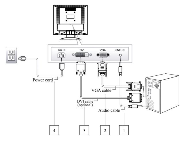
Figure.2. Connecting to a PC
